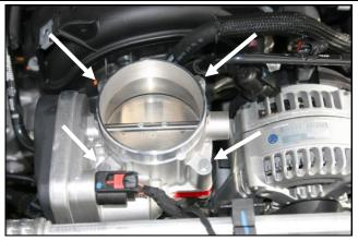
**5.** Reinstall the throttlebody on top of the Poweraid Spacer using the four bolts and the washers that were selected in step 3. Tighten the bolts evenly, in an X pattern, to the vehicle manufacturers specifications.
