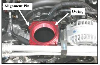
**4.** Install the supplied o-ring into the groove on the Poweraid Spacer. Next install the spacer onto the intake manifold with the o-ring facing up, making sure that the alignment pin holes are located over the alignment pins.
