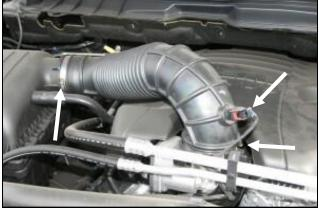
1. Disconnect the negative battery cable! Disconnect the air intake temperature sensor wiring harness by sliding the red tab, and then squeezing the black tab. Loosen two hose clamps, one on each end of the flexible air intake tube. Remove the tube from the vehicle. Lift straight up on the front of engine cover, pull it towards you, and set it aside.
